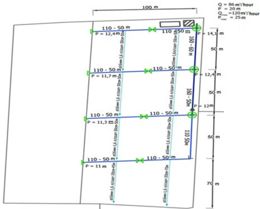
Fig. 1. Scheme of construction and division of sectors of the drip irrigation system
