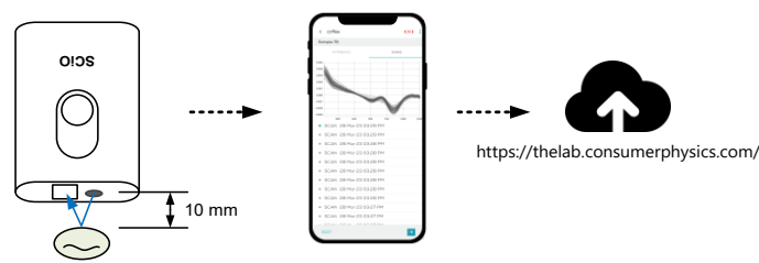
Fig 1. Scheme of data collection using a portable NIR spectrometer
