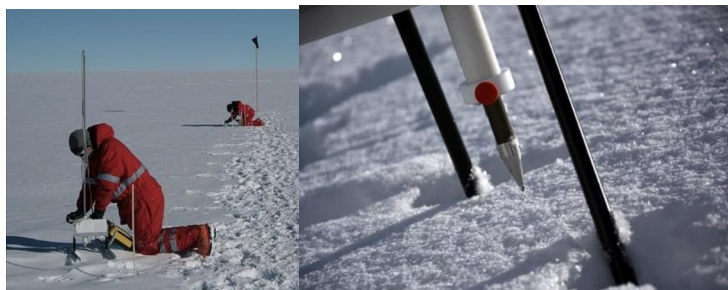
Fig. 4. Exterior view of Snow micro pen device operation (www.slf.ch/en)
