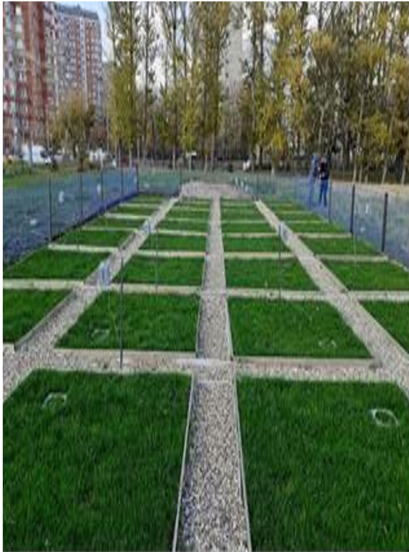
Fig. 3. The micro-plot field experiment with the bases of the over-ground exposure chambers.
