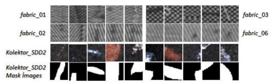
Figure 3 Examples of actual defect samples of size 32x32 pixel each, generated using both defect images and corresponding mask images provided by the AITEX and KSDD2 datasets.
