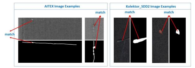
Mask images unambigiously define exact positions of the defects on the original samples
