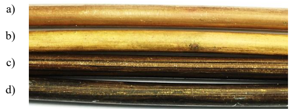
Fig. 2. View of the surface wires: a) fabricated, b) etched, c) annealed (200 °C/1h) and d) annealed (600 °C/1h)
