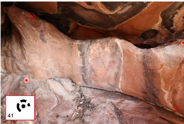
Figure 2: Location of the CPs (red dots) and sample image of the coded targets used inside the rock shelter.
