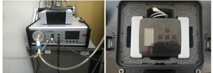
Fig. 2 Active radon detectors to be used in monitoring. The left figure is an AlphaGUARD while the right figure is the Rad Elec Recon detector.
