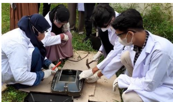
Figure 3. Process of Taking a CRT from a used TV tube
