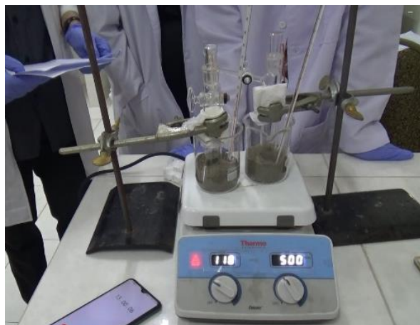
Figure 6. CRT Leaching Process in DES Extractant
