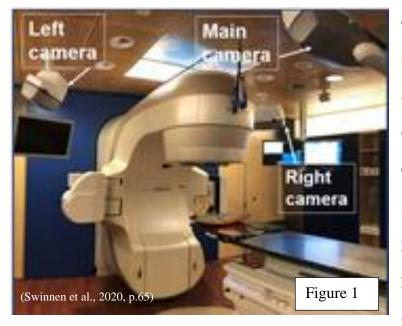
comprise of three ceiling-mounted scanner cameras arranged approximately 120 degrees to each other (Swinnen et al., 2020). The configuration of the cameras can be seen in Figure 1. The scanners project a light pattern over the patient's surface and are reflected and captured by the cameras,
