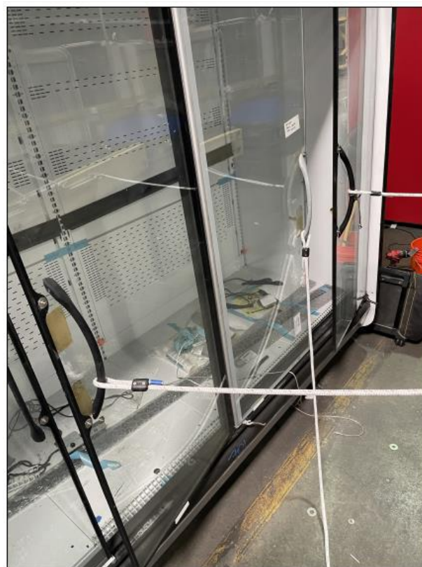
Figure 10: Rope attachments to cabinet door handles using rope clamps.
