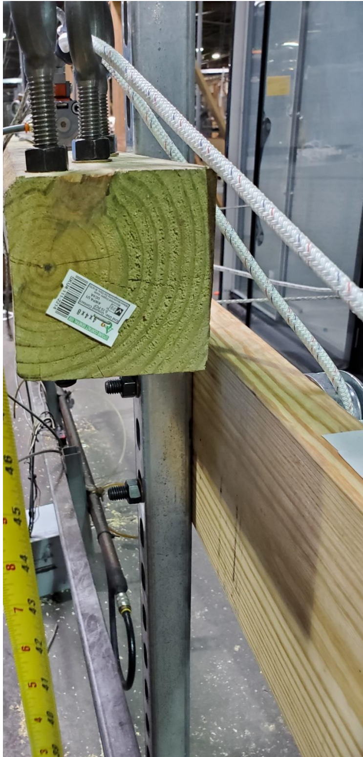
Figure 12: The structural board orientation.
