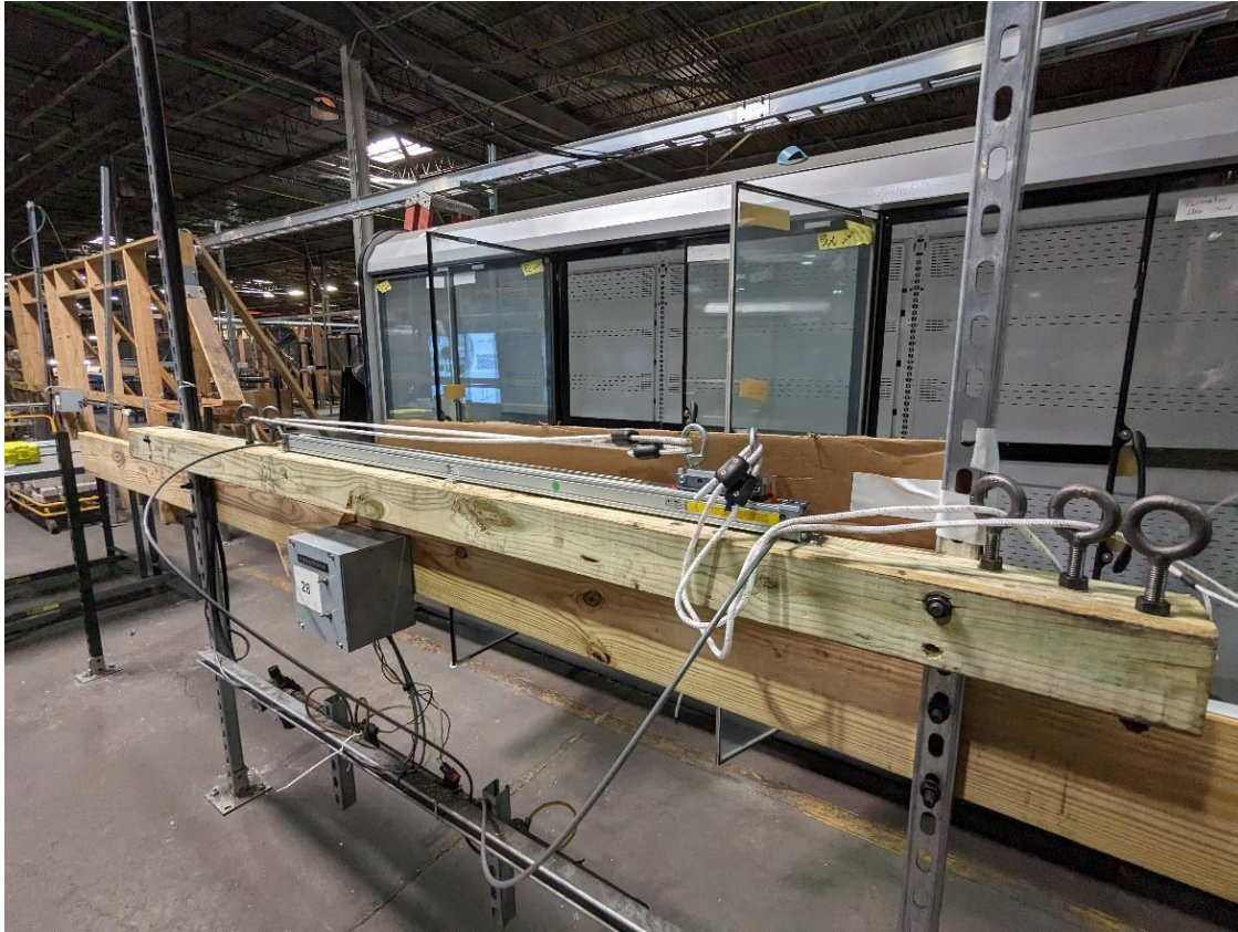
Figure 11: The cardboard was added to prevent the rope slack from catching on the pulleys.
