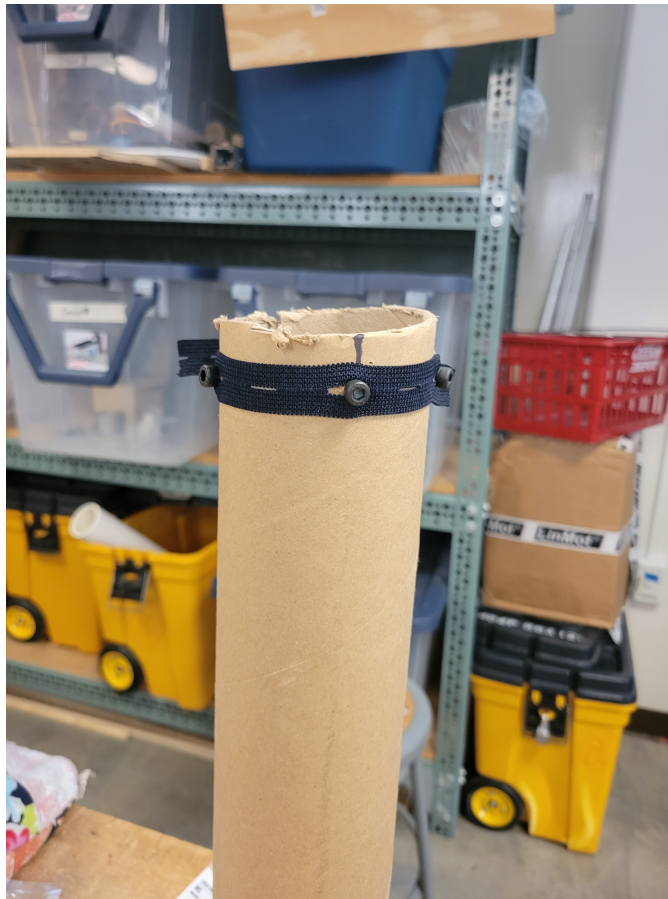
Figure 24: Proof of concept with an elastic band with holes in it from a children's pair of jeans around a cardboard tube.
