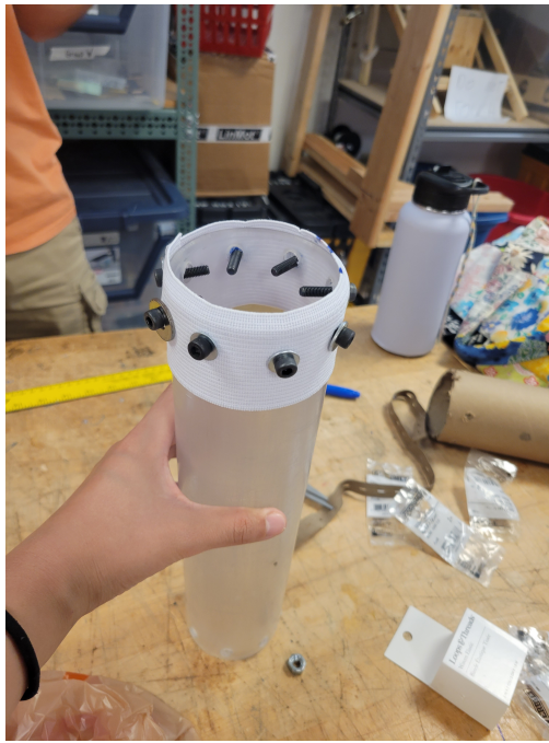
Figure 26: A photo of our first prototype showing our thicker elastic and pins.
