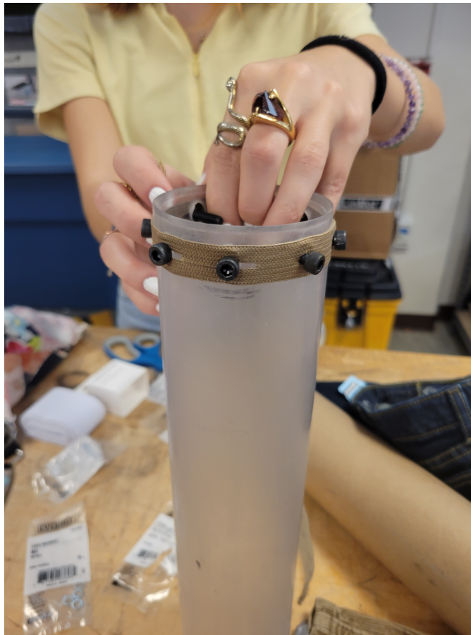
Figure 25: Proof of concept with an elastic band with holes in it from a children’s pair of jeans around the actual plastic tube.
