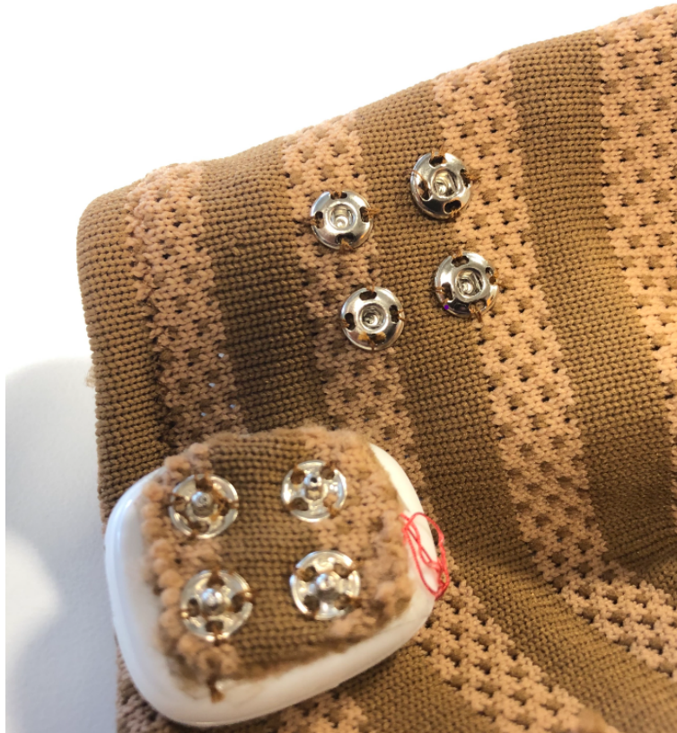
Figure 3: MIT E-TeCS Battery Connection
