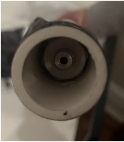
Figure 33: Pressure gauge inside PVC shaft.
