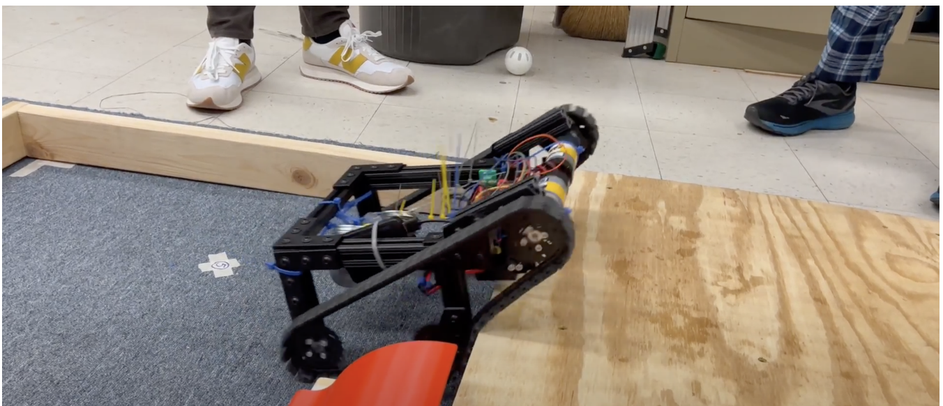
Figure 27: The robot attempting to complete Prototype Performance Goal 2 (traversing a piece of plywood).
