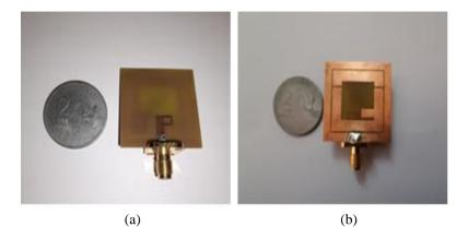
Fig. 2 Top (a) and bottom (b) view of the fabricated antenna
