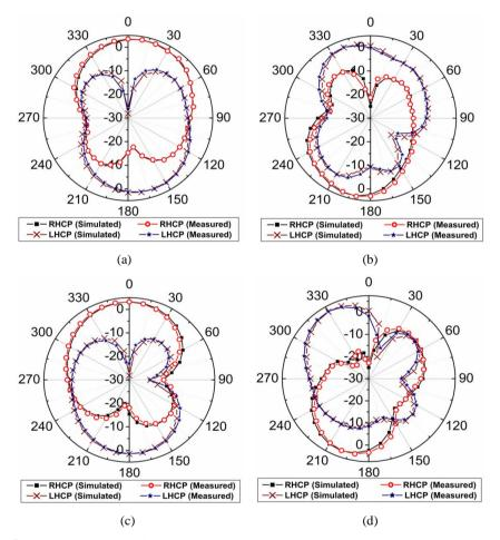
Fig. 5 Radiation pattern of the proposed CP antenna in the x-z plane at (a) 4.96 GHz; (b) 11.4 GHz and in the y-z plane at (c) 4.96 GHz (d) 11.4 GHz
