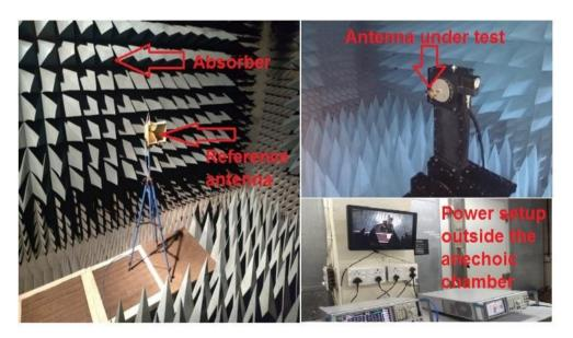
Fig. 6 Measurement setup for gain, axial ratio and radiation pattern of the proposed antenna in anechoic chamber
