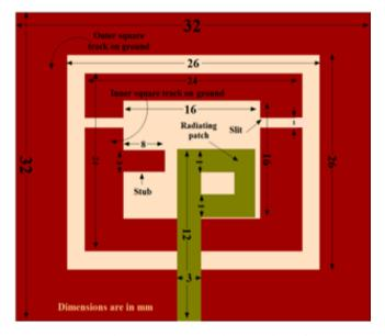
Fig. 1 Geometrical top (green color) and bottom (red color) view of the proposed structure
