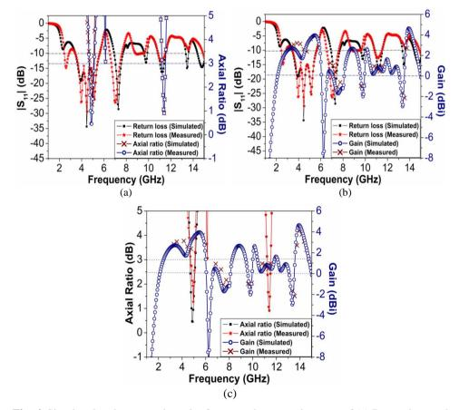
Fig. 4 Simulated and measured result of proposed antenna in terms of (a) Return loss and axial ratio; (b) Return loss and gain; (c) Axial ratio and gain
