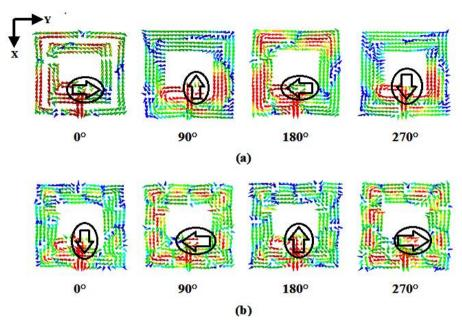
Fig. 7 Surface current distribution with 90° phase shifts for (a) 4.96 GHz; (b)11.4 GHz.
