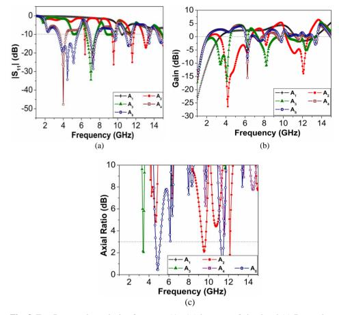
Fig. 3 Top Parametric analysis of antenna (A<sub>1</sub>-A<sub>5</sub>) in terms of simulated (a) Return loss; (b) Gain; (c) Axial ratio
