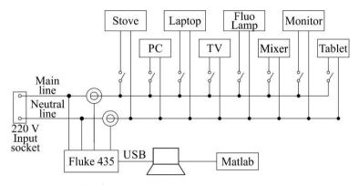
Fig. 4. Schematic of the experimental setup
