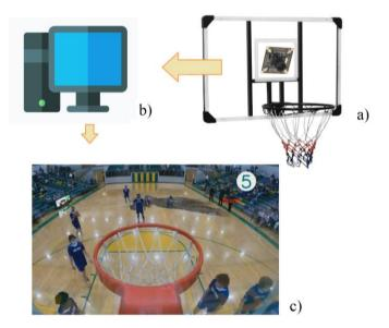
Fig. 1 Functional scheme of Vision Based Basketball Score Tracking System: a) Image aquisition using 2MP camera module with the wide-angle lens; b) Data processing; c) Output results presented within the camera view
