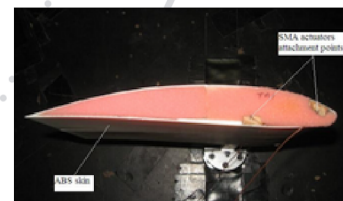
An aerofoil embedded with SMA for morphing ability [4]
