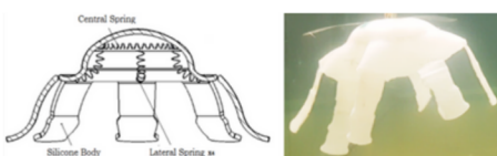
Jellyfish soft robot using SMA spring as actuator [1]
