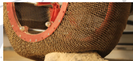
The Mars SMA Spring Tire developed by NASA [3]
