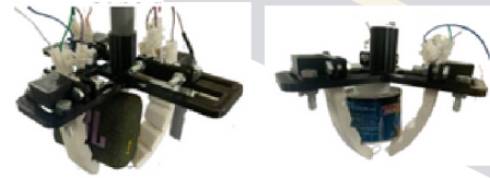
SMA-based soft gripper developed by this author [2]
