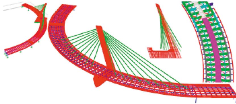
FIGURE 9: Finite element model of the curved composite stay-cabled bridge, the Marghera bridge.
