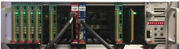
Fig. 92 WaveDREAM crate shown with 7 WDB (green), one ancillary board (red), one TCB (blue) and the CMB (right)
