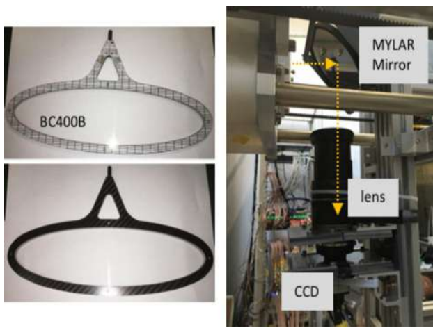
Fig. 18 (Left) shows two sides of the prototype PVT target used during the 2016 Pre-Engineering Run. The calibration grid is used for the perspective transformation. The carbon-fibre/Rohacell ® foam frame can be seen from the other side. (Right) shows the CCD setup and Mylar mirror at the downstream side (DS) of the COBRA magnet \sim 2.1 m DS of the target
