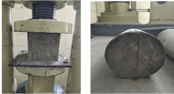
Fig. 5 Testing of cube and cylinder
