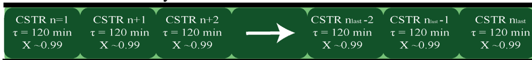
FIGURE 3 Switch flow technique, after achieving steady state conditions at a fast flow rate, the pumps are lowered. Achieving a complete conversion profile because every fluid element has a defined residence time in the reactor
