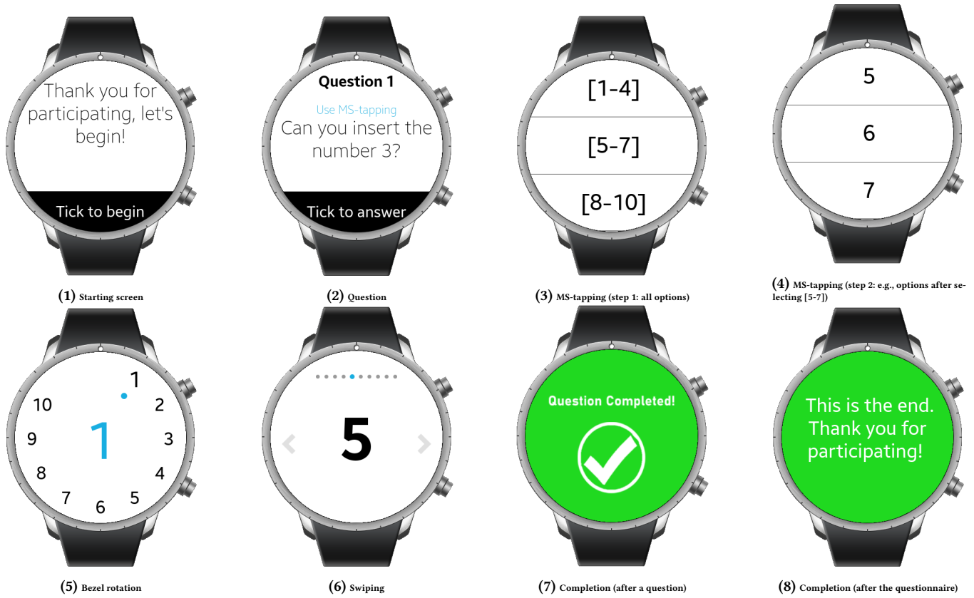
Figure 2: Screenshots of the smartwatch application guiding participants through the study procedure and implementing the three input techniques we compare
