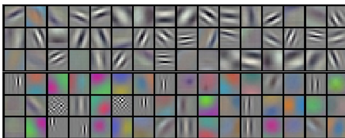
Figure 2.8. Filters learned by one of the layers of the AlexNet architecture. It can be observed that these filters are similar to the basis functions of the DTCWT depicted in Fig. 2.2. Image from Krizhevsky et al. [5].
