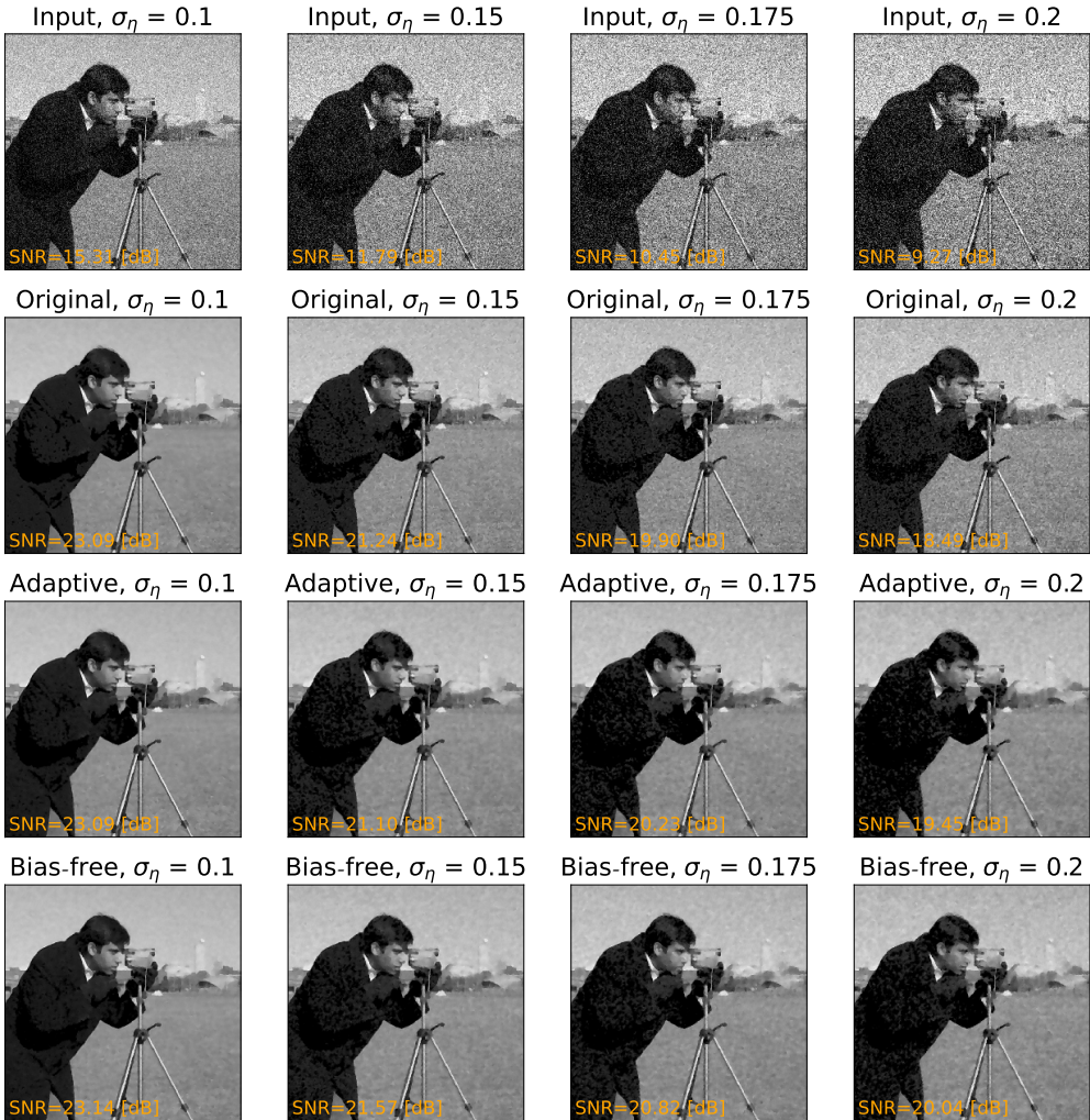
Figure 3.13. Comparison of the baseline (original) toy model against its adaptive and bias-free variants. The models are evaluated in the cameraman picture with increasing noise levels. The top row displays the noisy input. The second top-row represents the images processed with the original toy model. Meanwhile, the third row are the results of the adaptive toy model. Finally, the bottom-row are the results corresponding to the bias-free model. It can be observed that the performance original toy model degrades as the noise level increases, while the performance adaptive and bias-free model degrade less with increased noise levels, resulting in pictures with lower noise levels.
