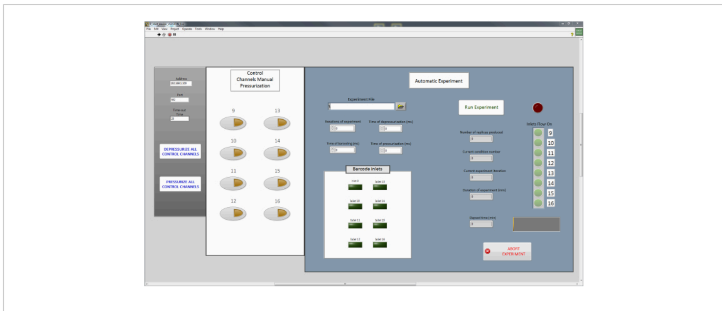
Figure 3: The main interface program to control the microfluidic device. This custom-made program enables manual pressurization of individual pneumatic valves (white panel). It also allows the execution of a complete experiment (blue panel) where it accepts a .csv file with the desired plug populations and necessary parameters such as valve pressurization and depressurization times and displays the status of the experiment execution, including which control channels are pressurized and not, in real-time. Please click here to view a larger version of this figure.
