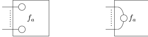
Figure 5.7: Mean field (left) and joint (right) factorisation constraints for variable numbers of edges on a CFFG.
