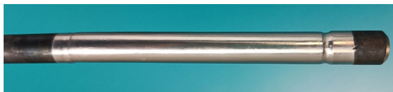
Figure 1. Picture of prepared Pd–Ag membrane (M2) for SMR studies.
