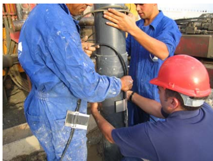
Fig 3. Attaching downhole electrodes to borehole
