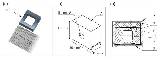
**Fig. 2** Design of cesium MEMS cell and heating assembly. (a) Photograph of cesium MEMS cell with 3 mm optical path. (b) Drawing of the external cell oven assembly. (c) Cross-section of oven, insulation and cell. A: 3D printed cell housing, B: calcium-magnesium silicate thermal insulation, C: t-type thermocouple, D: cesium 3 mm MEMS cell, E: non-inductive SMD resistor, F: heater interface PCB.
