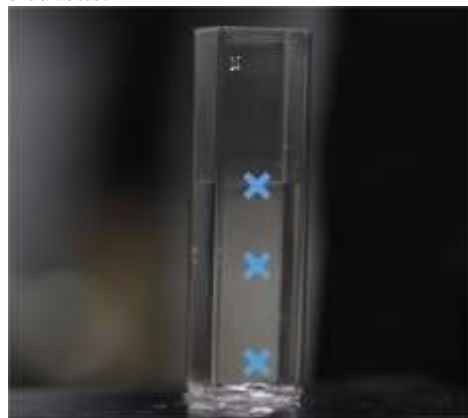
Fig. 2. The three points on the cuvette in which the dynamics of temperature change is observed.
