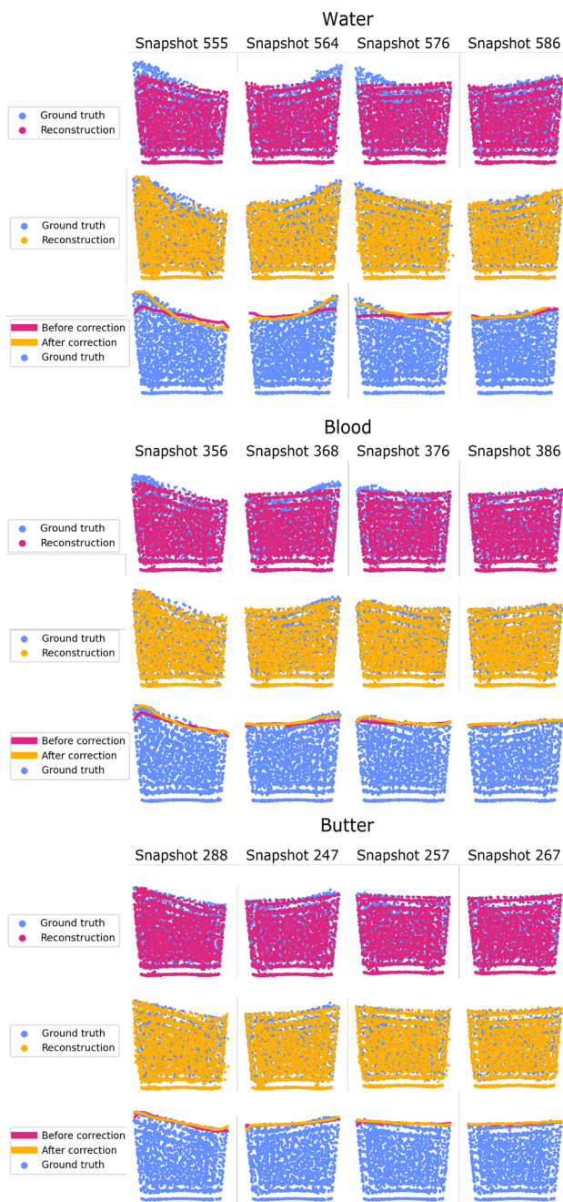
Fig. 5 Fluid reconstruction before and after correction of water, blood, and butter. Representation of the sloshing peaks of ground truth (in blue) compared to the network results before (in red) and after (in yellow) applying the correction to adapt to observations in selected critical snapshots, indicated in the figure. (Color figure online)
