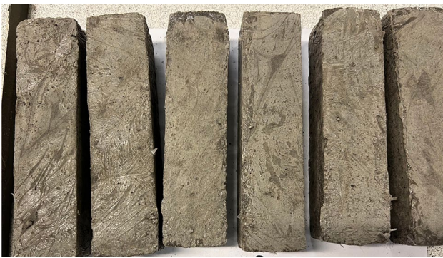
Fig. 3 Prism mortar samples after demoulding
