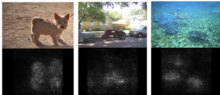
Figure 2.5: Examples of the produced saliency maps using a single back-propagation pass through a ConvNet classification neural network [86].
