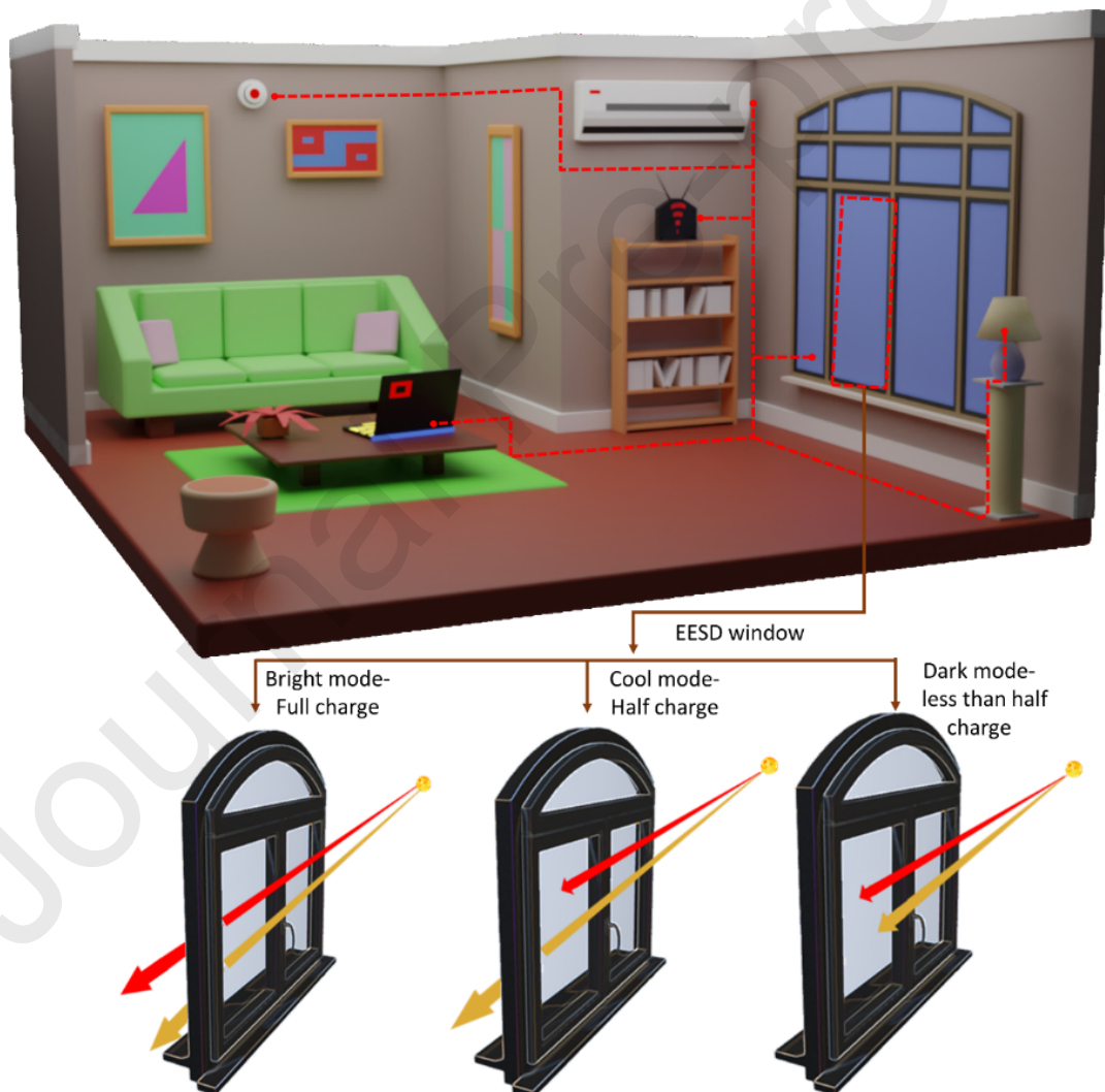
Figure 18. Energy distribution in powering different devices in room (alarm sensors, portable components, controlling heat and light) by EESD in day and nighttime using different charging conditions.
