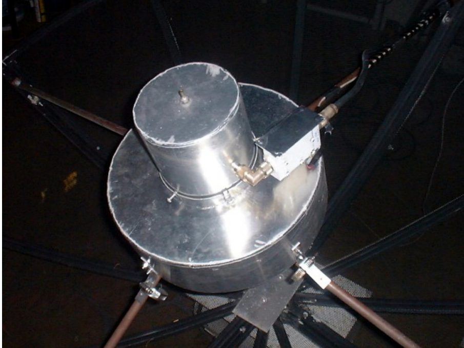
Figure 21: Example of a antenna and feedhorn provided by Radio Astronomy Supplies
