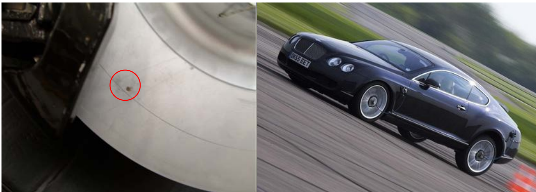
Figure 1: Thermocouple in Front Brake Disc and Test Vehicle Fitted with Slip Rings
