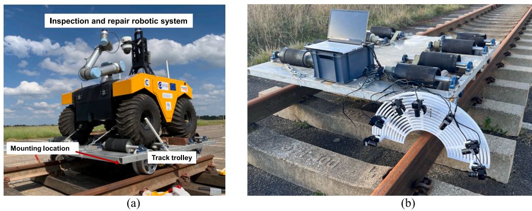
Fig. 12. (a) The robotic platform [43,44]. (b) System integration on the front base trolley.
