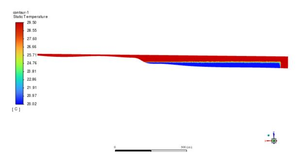
Figure 9. Model 2 temperature contour of initialized stratification.
