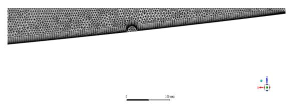
Figure 8. Model 1 mesh display, zoomed in to inflation layers on bottom boundary.
