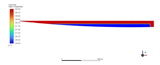
Figure 7. Initialization of Model 1 with temperature and salinity values in Ansys Fluent. Temperature contour of ZX axis in middle of domain at y=500.
