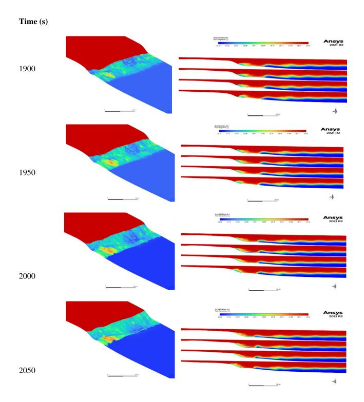
**Figure 16.** Temperature contours of bottom surface (left) and ZX planes spaced 100 m apart along the Y axis (right). Sequential images every 50 timesteps from internal bore propagation, run-up, breaking and receding along the reef slope.
