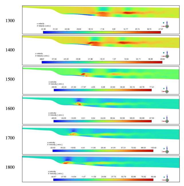
**Figure 17.** Model 2 contours of X-Component of velocity (cm/s) shown on ZX plane in middle of domain for timesteps 1300-2400.
