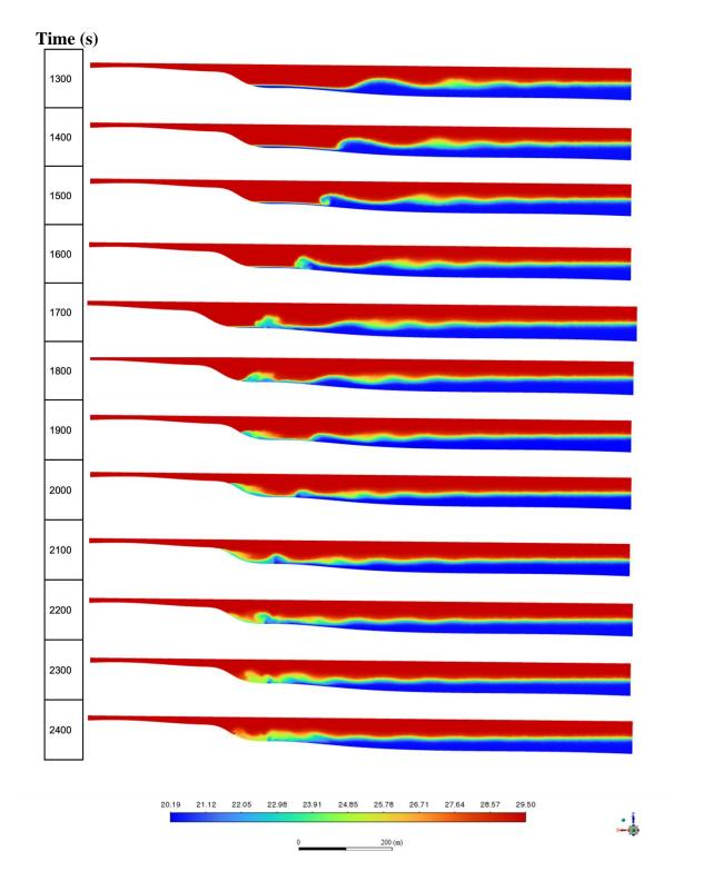
**Figure 15.** Model 2 temperature contours on ZX plane in middle of Y-axis of the domain. Internal waves traveling along the thermocline can be seen propagating (from the right) towards the slope, breaking, and receding throughout the simulation. Images taken every 100 timesteps (100 s) throughout the calculation.
