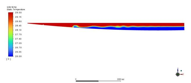
Figure 12. Model 1 temperature contour on ZX plane at timestep 4000. Leading wave begins to overturn and break on steepening slope.
