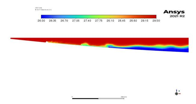
Figure 13. Model 1 temperature contour on ZX plane at timestep 5530. Bore run-up to hypothetical reef structure.
