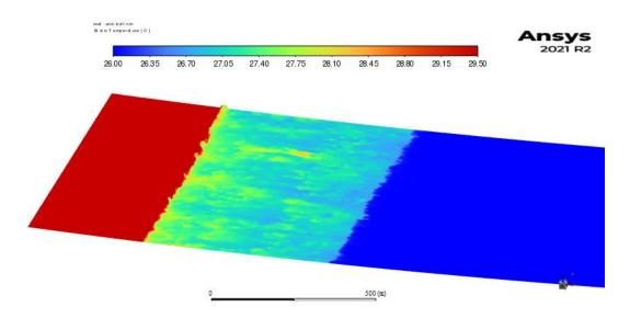
Figure 14. Model 1 temperature contour on bottom boundary and reef structure at timestep 5530. Bore run-up to hypothetical reef structure.
