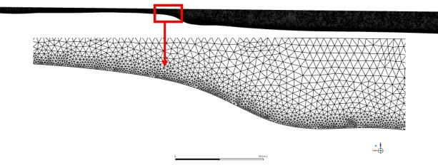
Figure 10. Model 2 Mesh display, zoomed in on reef slope to show smaller mesh on bottom boundary.
