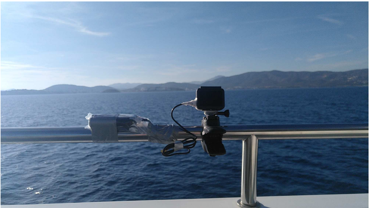
Figure 31: GoPro installation on the SOCIB vessel railing. The GoPro in its clamp can be seen at the right, the power-bank can be seen to the left. Cables and connections are waterproofed as much as possible using plastic bags and tape.
