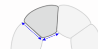
Cell Aspect Ratio Major cell axis divided by minor cell axis length
