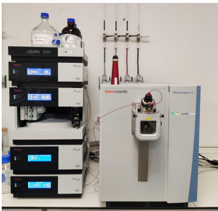
Figure 12. Thermo Scientific HPLC (Dionex UltiMate 3,000 series, Thermo Scientific - San Jose, CA, USA) equipped with a diode array detector (DAD) and connected in series to an Orbitrap mass spectrometer (MS, Exploris 120, ThermoFinnigan - San Jose, CA, USA).
