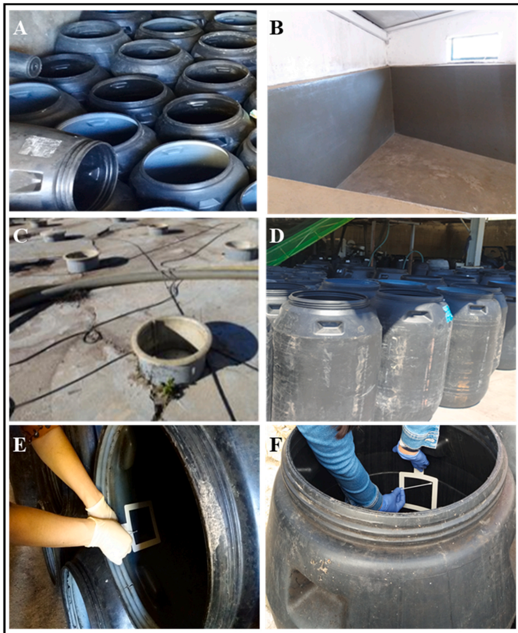
Fig. 1. Photograph of the table olive fermenters (A, B, C, D) and microbiological surfaces sampling by the swab contact method (E, F).
