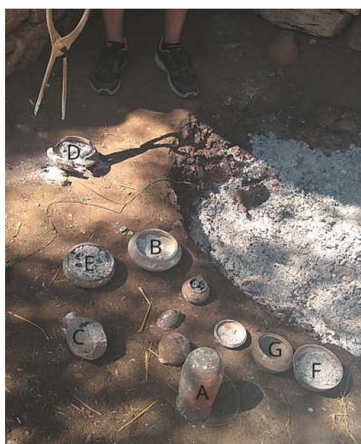
Figure 5. Vessels extracted from the pit, post firing. Vessel C lost its outer layer, Vessel D failed, and Vessel F cracked; the rest of the vessels survived the firing.
