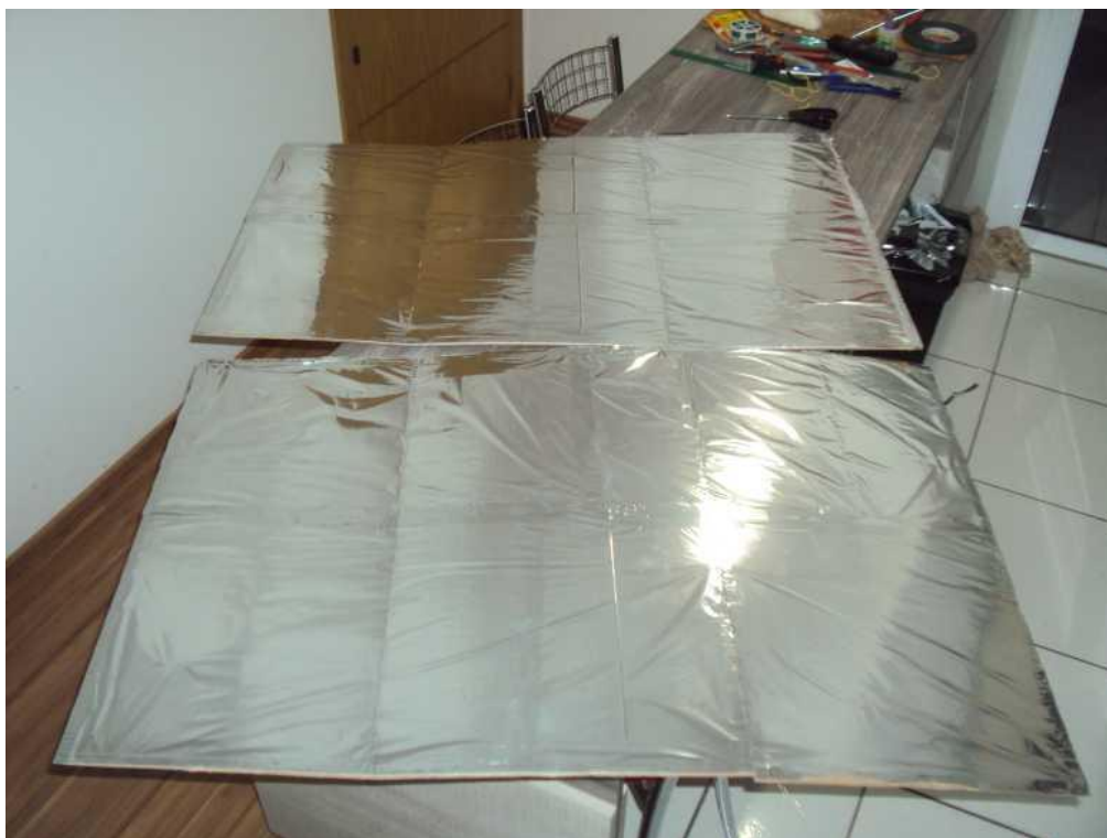
Figure 12 – Two cardboard sheets covered with reflexive films. Source: The authors
