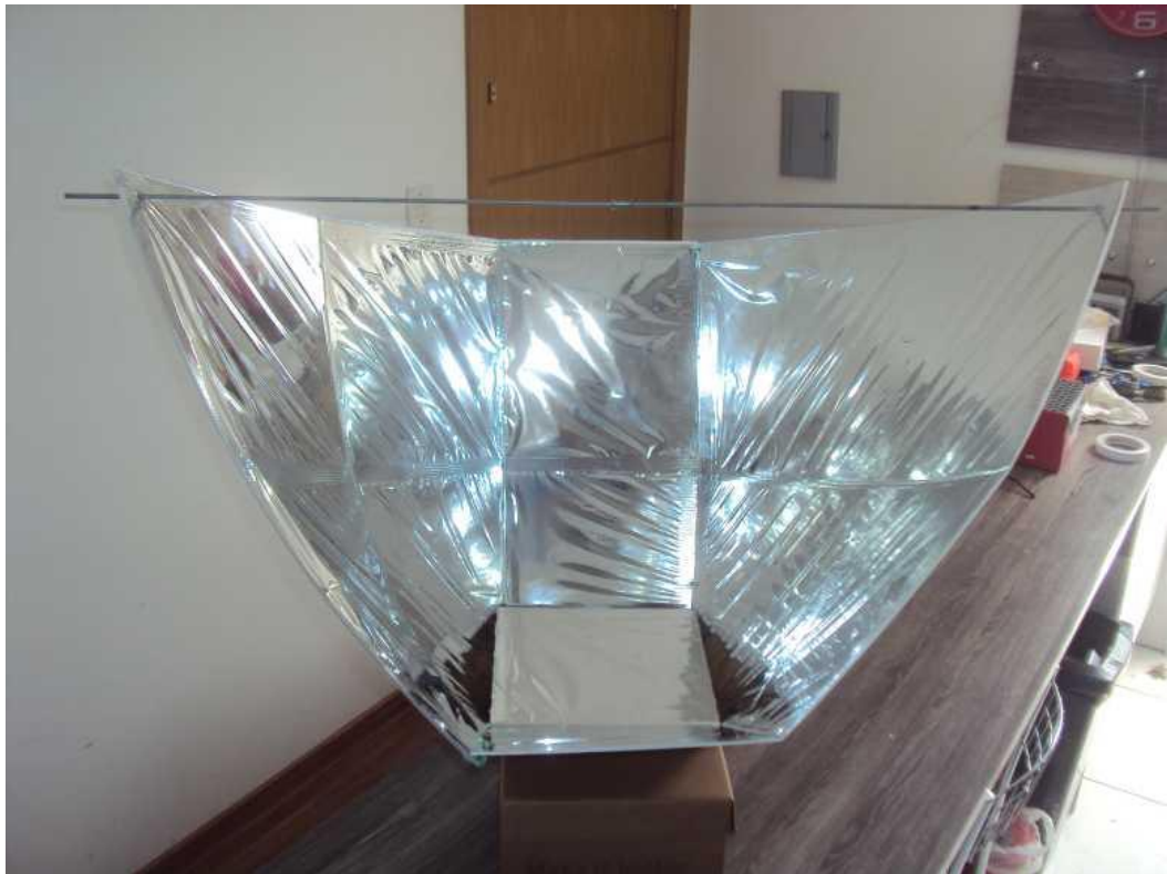
Figure 13 – An assembled, ready-to-use Fun Panel solar cooker manufactured in the Morro da Cruz Workshop. Notice the shoes box used as pan support. Source: The authors
