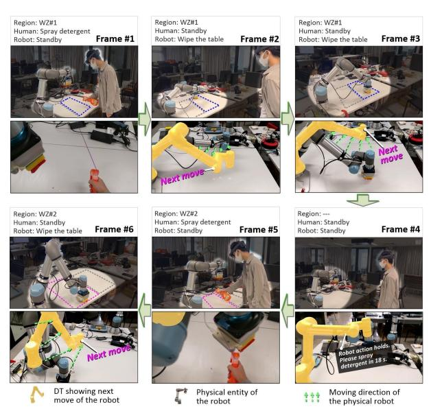
**Fig. 10.** Implementation results of OTCM, which predicts and visualizes robot movements to guide the human co-worker (Note: the top and bottom row in each frame represent the thirdperson and the HoloLens view, respectively).
