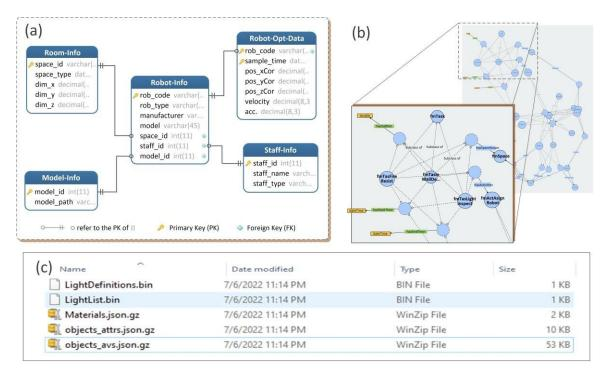
**Fig. 5.** Database server composition: (a) Entity relationship diagram of the database; (b) Graph representation of the knowledge base; (c) Models stored on the database server as separate files.
