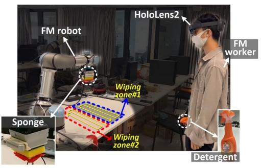
Fig. 9. Setup of the table disinfection task in Scenario #2.
