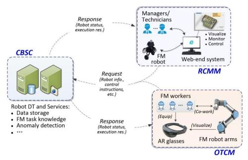
Fig. 4. Architecture of the system prototype.
