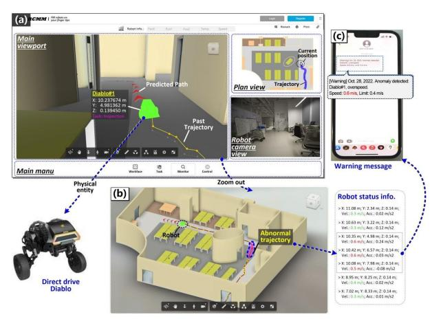
**Fig. 8.** Implementation results of the RCMM: (a) Web interface of the module; (b) Zoom-out showing the moving trajectory of the inspection robots; (c) Warning message received on mobile phone about abnormal robot operation, e.g., overspeed.
