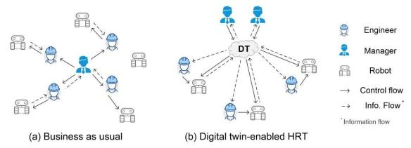
**Fig. 2.** Schematic diagrams showing how FM robots are teamed up with their human peers (a) in existing practice, and (b) in a DT-enabled model.
