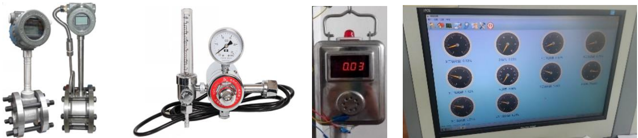
(a) Vortex flowmeter (b) CO 2 decompression valve (c) CO 2 sensor (d) Data acquisition platform
