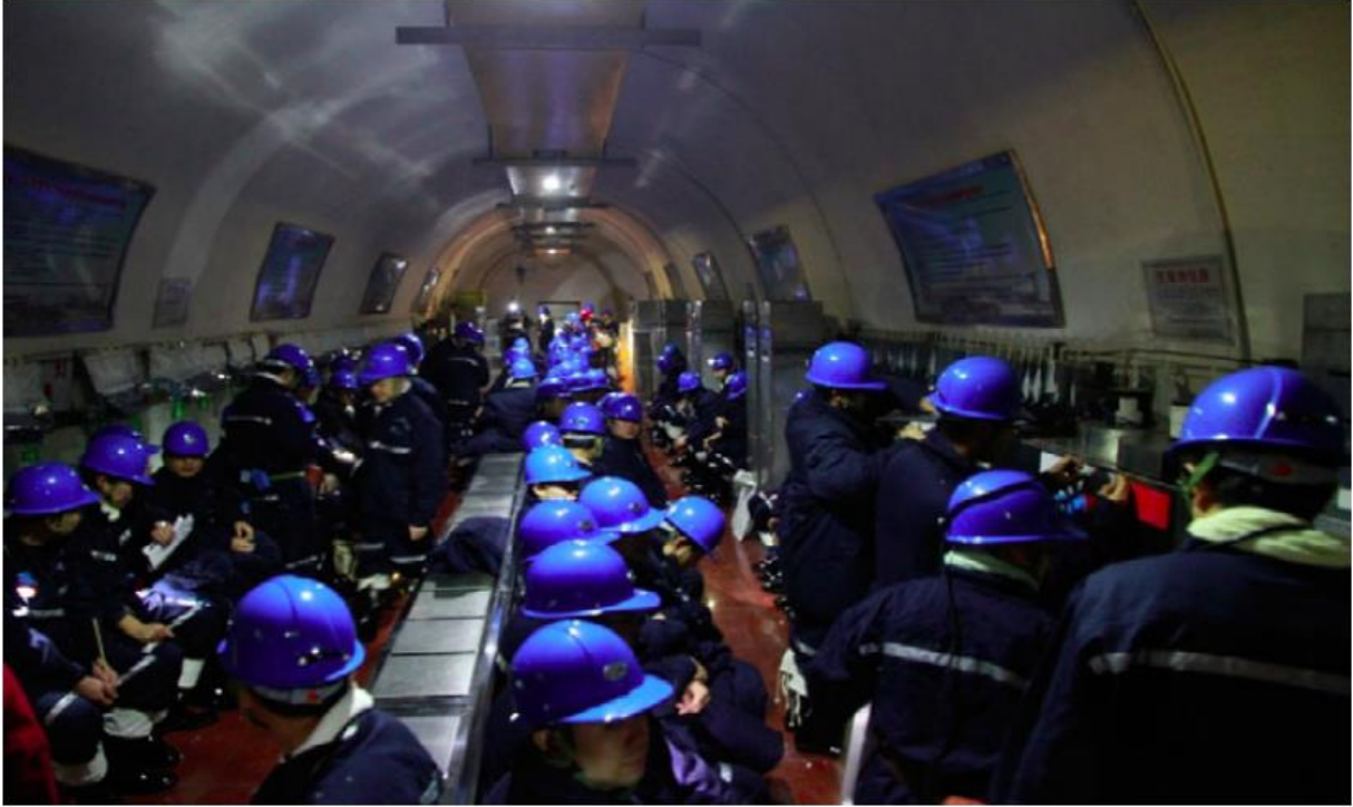
Fig. 1 Experimental scene of air quality control for 80-person MRC by ventilation. [36]
