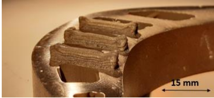
B) Sample of GTD 111 printed by LP-DED
