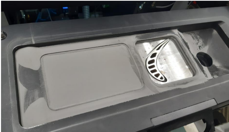
Figure 29. Inside of L-PBF machine at OSU
