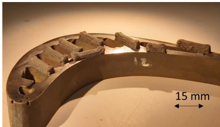
C) Sample of GTD 111 printed by LP-DED
