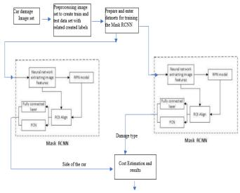
Figure 1: Detection of Car-damage and cost system framework
