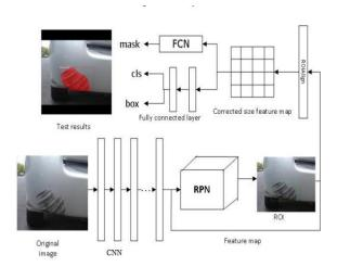
Figure 2: The framework model of Mask RCNN (Kalpesh Patil, Mandar Kulkarni,2017)
