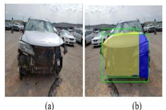
Figure 9. Damage localization. (a)Original front crash image, (b) The result of Mask RCNN (green box). Note that our proposed approach is capable to find the size and localize the area of the damage correctly.
