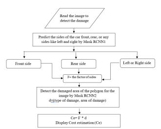
Figure 8. Flowchart of the cost estimation process
