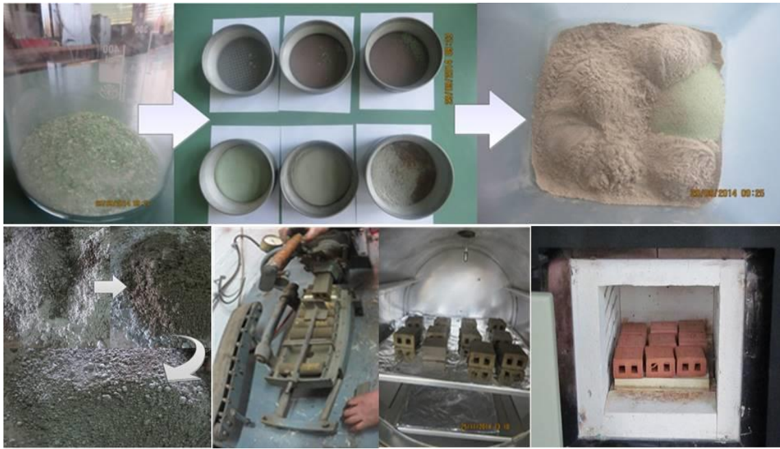
Figure 2. Phases of obtaining experimental clay blocks with waste glass
